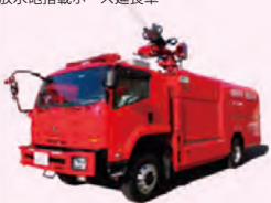
Hose extension car equipped with large water cannon 大型放水砲搭載ホース延長車
