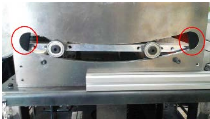
Fig.2 Side view of the pendulum tilting table which cushioning materials attached
