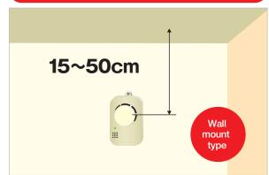
Note: The center (sensing parts) of the residential fire alarm should be located between 15 to 50 cm of the ceiling.
