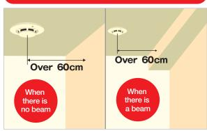
Note:Install the residential fire alarm by keeping a distance of 60 cm or more between its center (sensing parts) and the wall. If there is a beam on the ceiling, keep a distance of 60 cm or more between the center of the residential fire alarm and the beam.
