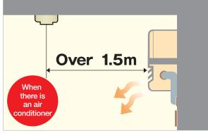
Note: Keep a distance of 1.5 m or more around the exhaust area of an air conditioner or ventilation fan.
