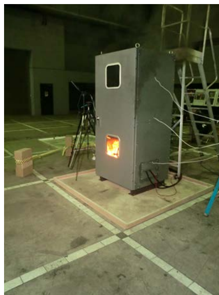
鉛蓄電池延焼状況②
