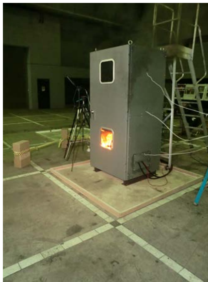
鉛蓄電池延焼状況②
