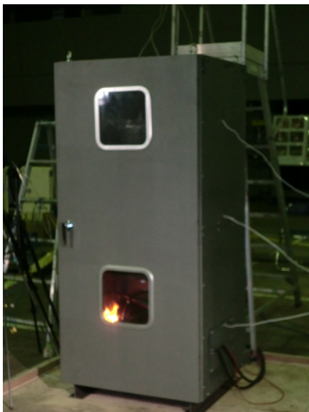
鉛蓄電池延焼状況①
