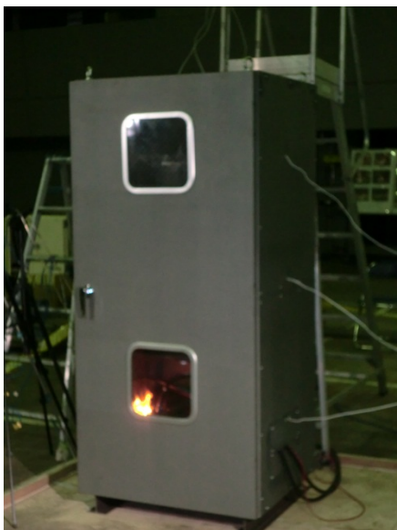
鉛蓄電池延焼状況①
