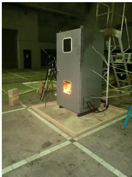
鉛蓄電池延焼状況②
