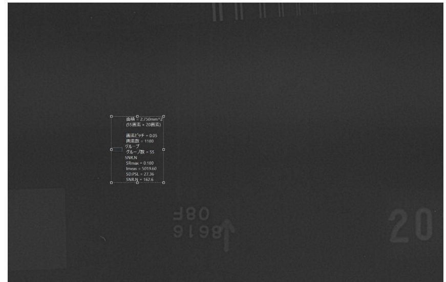
板厚 36mm D-RT (CR) SNR_N 確認例
