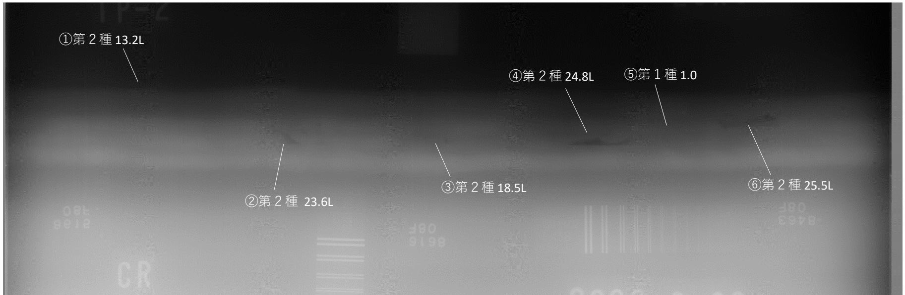
TP-2 板厚 28mm x 38mm 突合せ溶接試験片 D-RT (CR [IP] )
