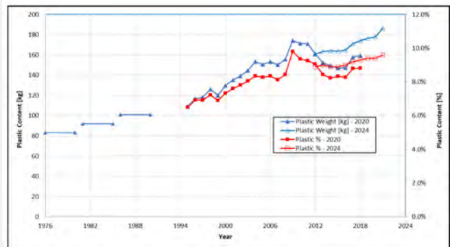
Figure 10. Vehicle plastic weight and weight percentage as a function of time (data source: American Chemistry Council, 2023)
