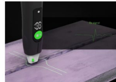
Figure 2: Illustration of the interaction between a crack and the induced eddy currents
