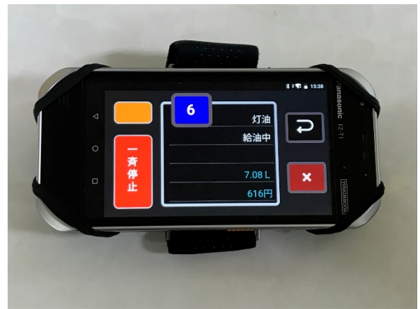
可搬式制御装置（給油中）②
